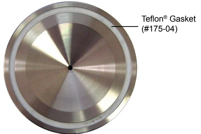
2. Pour the fluid sample into a clean aging cell to within one-half inch of the lip. This will allow sufficient void space for the expansion of the fluid due to heating. Avoid getting fluid on the lip of the test cell.
